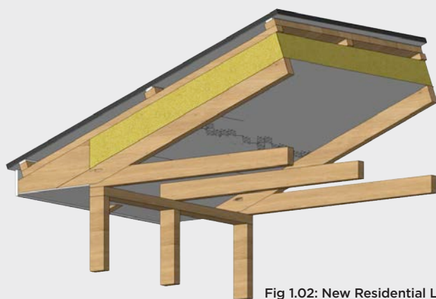
Fig 1.02: New Residential Longrun roofing - Trussed or Skillion
