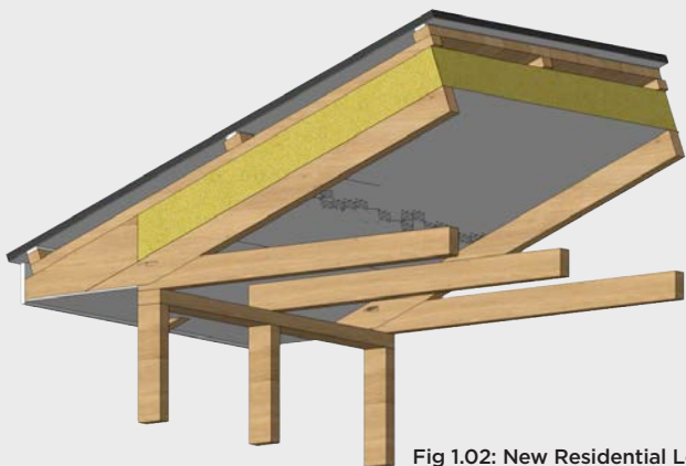
Fig 1.02: New Residential Longrun roofing – Trussed or Skillion
