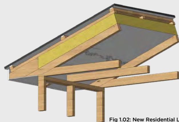
Fig 1.02: New Residential Longrun roofing – Trussed or Skillion
